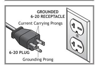
Figure 2. NEMA 6-20 plug & receptacle.
